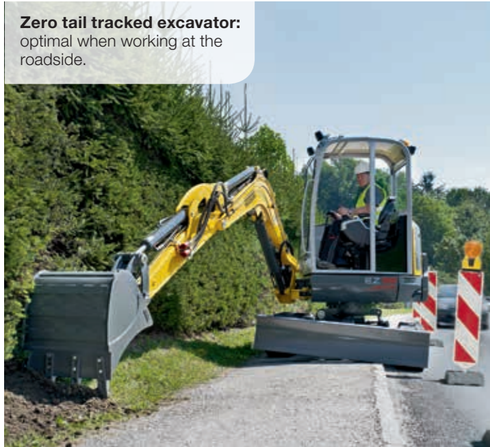
When there is not much space, the 803 - the smallest tracked excavator from Wacker Neuson - is ideal.
