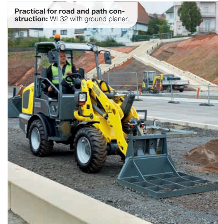
Two sturdy lift cylinders make a safe lift motion of the load arm possible.
