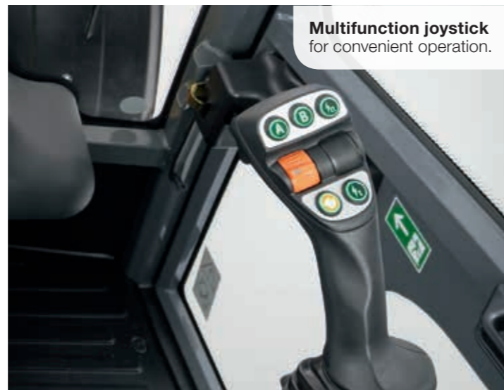
Adjustable joystick console moves jointly with the operator's seat
